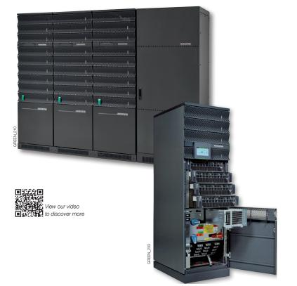
With its flexible modularity providing seamless and risk-free power scalability up to 600 kW, the MODULYS GP range is the ideal solution for unscheduled site upgrades or incremental power evolutions. The installed power can be increased up to 600 kW by adding hot-swap plug-in power modules for incremental steps of 25 kW.
