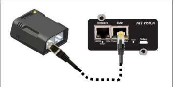
Connect a CAT5 Ethernet cable from NET VISION "EMD" connector to port on the EMD.
