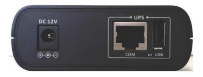
The serial link to UPS is located on the back of the box. The serial cable included in the package has to be connected to 'COM' RJ45 connector and to the UPS RS232 DB9 serial port. The UPS serial COM port used for NET VISION BOX has to be set as following:
